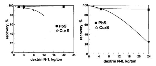
Fig. 4. Results of flotation of galena and chalcocite in the presence of dextrins N-1(a), and N-8 (b). pH = 7.1-7.2. Minerals were floated separately
