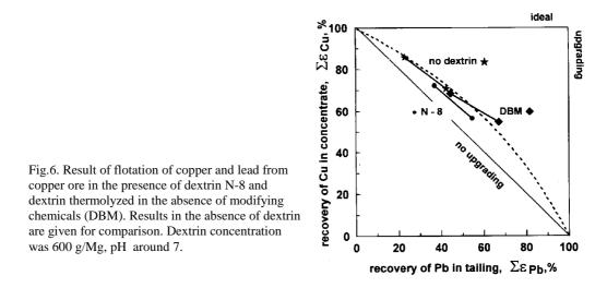
According to Lekki (2002) the reason of the unequal selectivity of separation achieved for synthetic mixtures and real ore most likely results from different redox environments in the systems.
